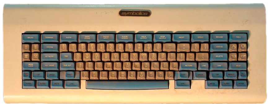
The Space Cadet keyboard from a Symbolics Lisp machine: a mixture of familiar and unfamiliar keys.
